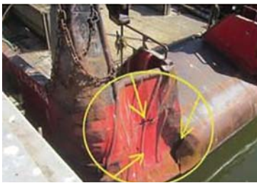
Collision damage to fishing vessel
